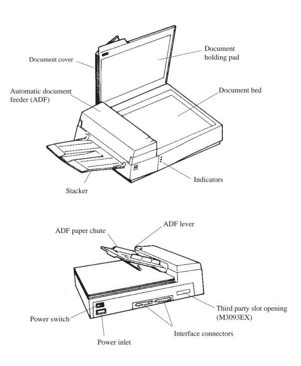
Figure 2.2 M3093EX/GX parts names
